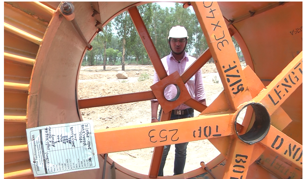
3 × 400 square mm 11 KV HT cable drum
